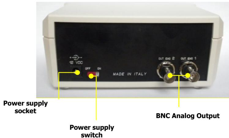
FIG. 2: EMG2 rear panel view
