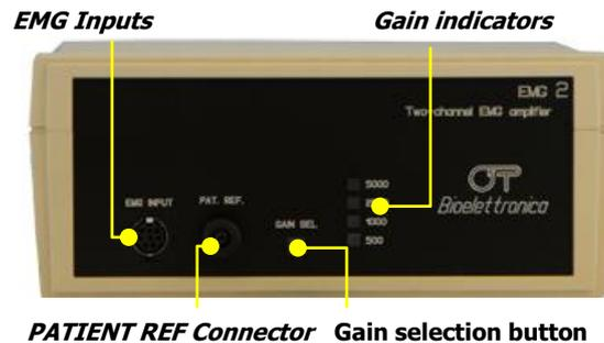
FIG. 1: EMG2 front panel
