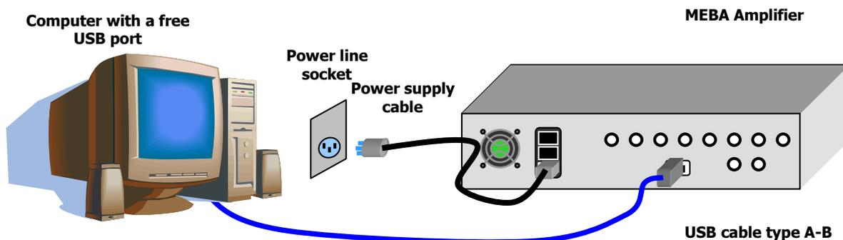
FIG. 5: Standard set up of the electromyograph
