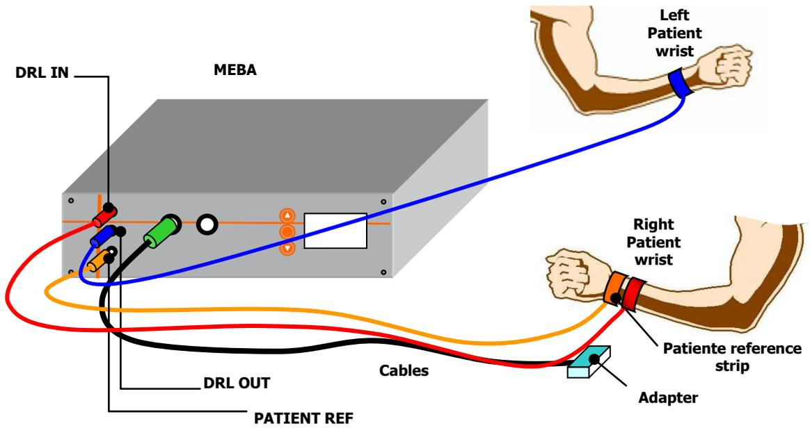
**FIG. 7:** Patient connection diagram for signal acquisition in floating monopolar modality
