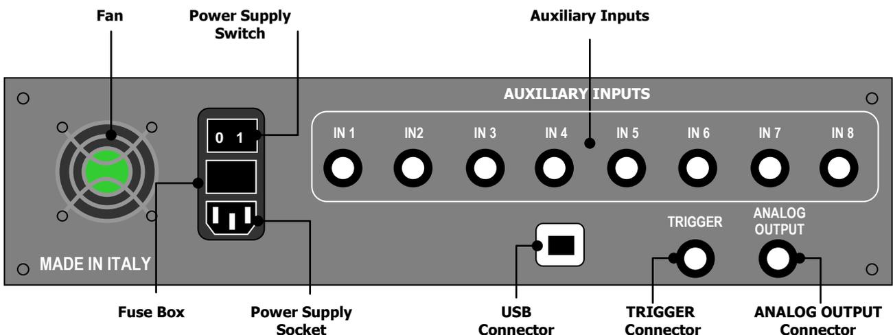
**FIG. 3:** MEBA rear panel view
