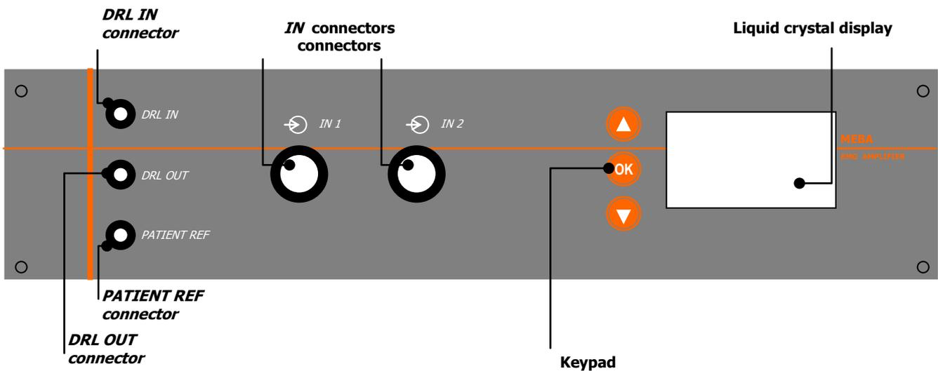
FIG. 1: MEBA front panel
