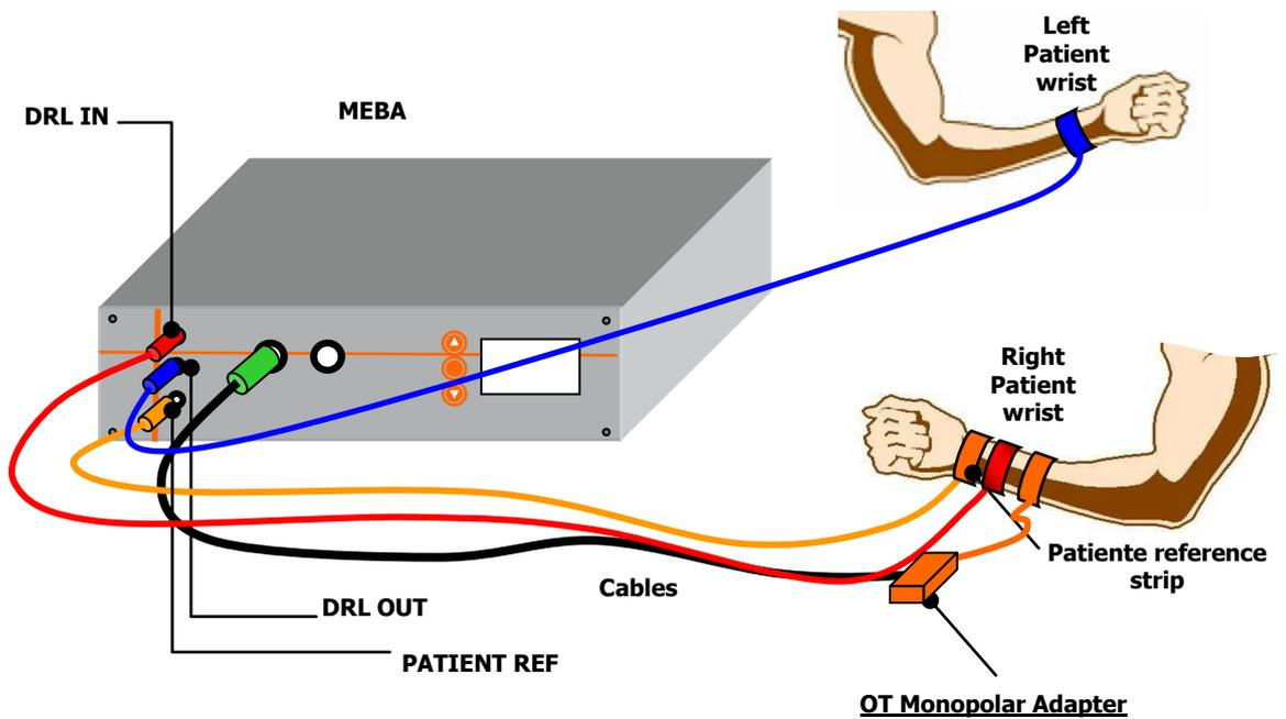
**FIG. 8:** Patient connection diagram for signal acquisition in referred monopolar modality
