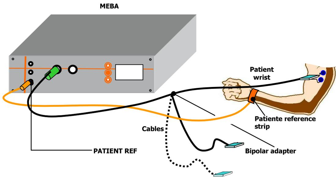
**FIG. 9:** Patient connection diagram for signal acquisition in bipolar modality
