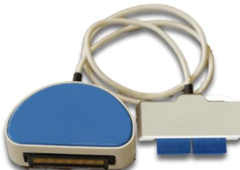
**FIG. 8.5:** *The AD1x16SE adapter*
